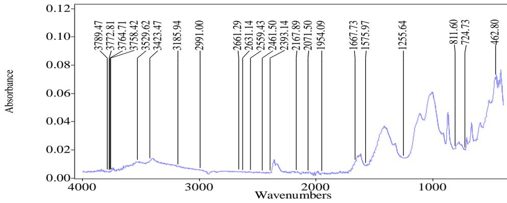
Fig. 12 FTIR spectrum (in the mid-infrared region) showing the use of animal glue as binding medium
