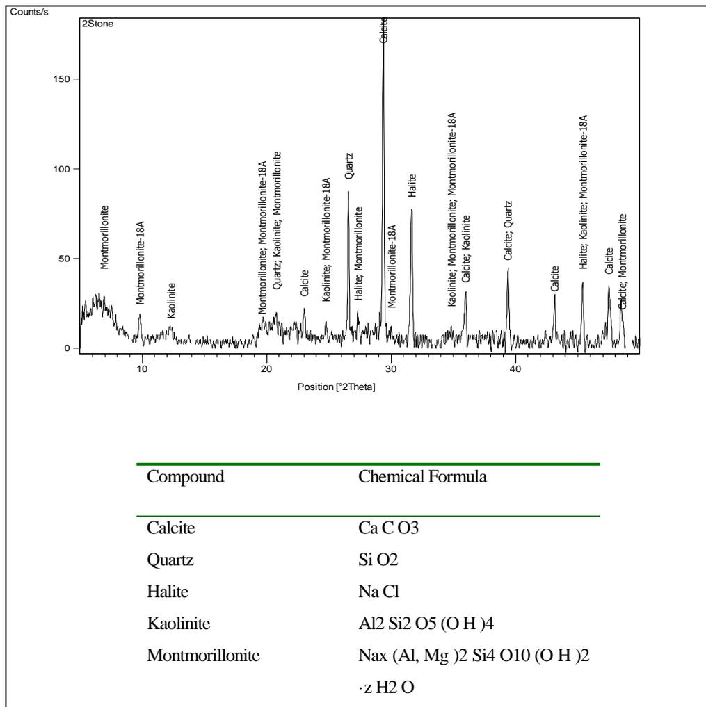
Fig. 6 XRD pattern and the main components of the bedrock, illustrating the presence of calcite and quartz, halite and clay minerals
