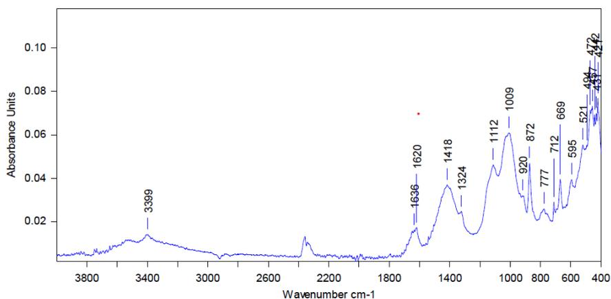
Fig. 11 FTIR spectrum (in the mid-infrared region) suggesting the use of a proteinaceous binding medium is probably animal glue
