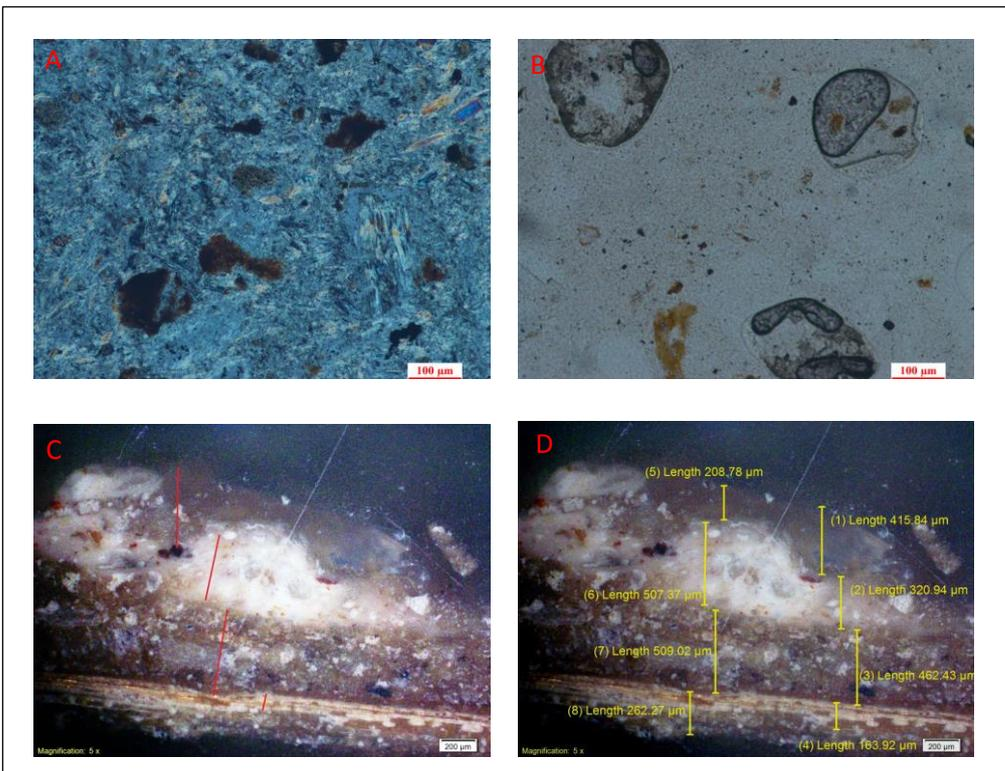
Fig. 8A-B The thin sections of the white mortar inspected with polarized light microscope (PLM) (The first layer in the bottom), the coarse layer revealing a main microfacies association and fossiliferous (Fig. 8C-D), the cross-sections on the plaster layers presenting a solid structure with differentiate three layers
