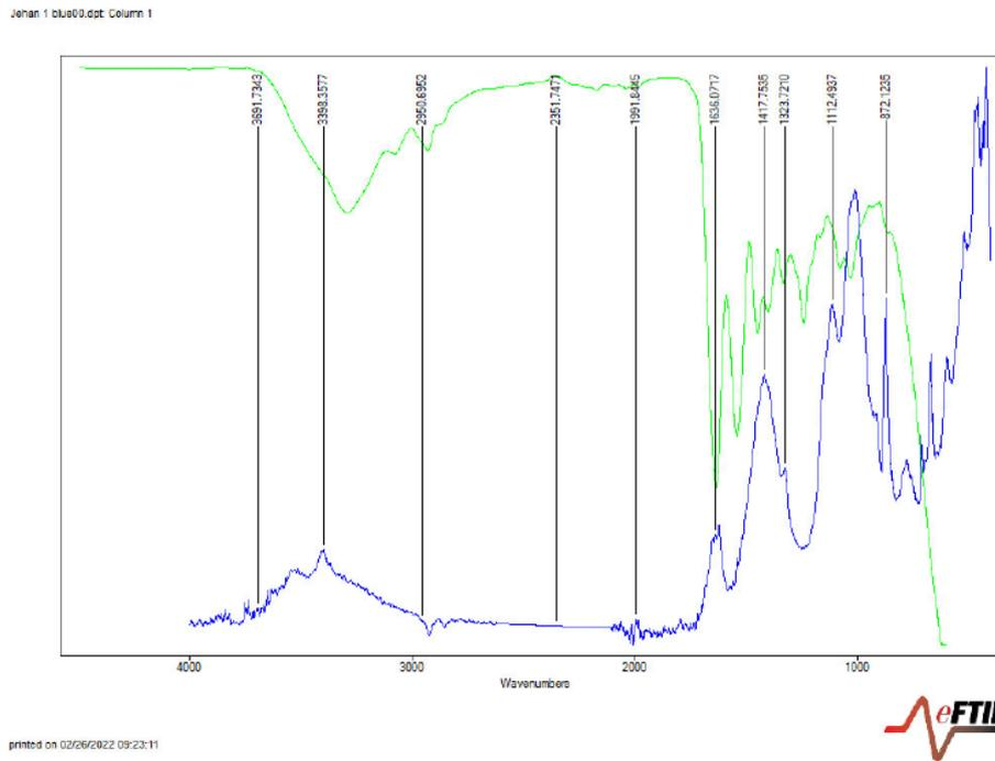
Fig. 13 FTIR spectrum (in the mid-infrared region) plaster layer, compared with a reference spectrum of animal glue
