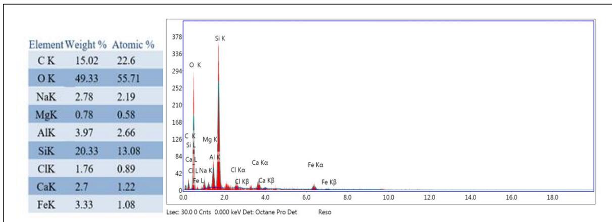
Fig. 10 The EDX analysis of the mortar sample showing that silicon, calcium, and aluminum are the major ions contained, while sodium, sulfur, iron and chlorine are the secondary elements, and traces of magnesium
