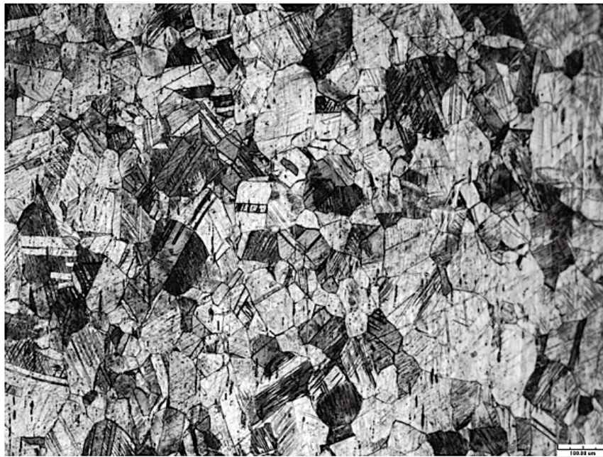
Figure 10. Metallography graphic of tube fitting with cryogenic treatment (100 \times ).
