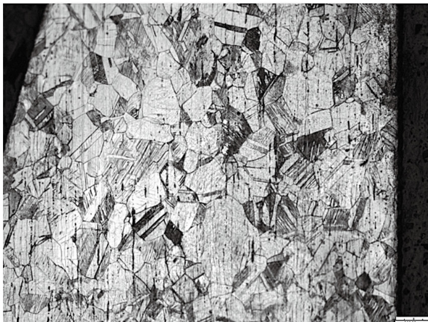
Figure 9. Metallography graphic of tube fitting without cryogenic treatment ( 100\times ).
