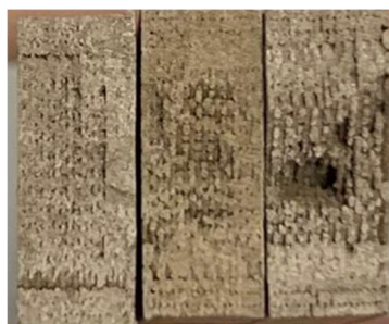
Figure 4: Results of the tensile teste, each print speed is 30(left), 60(center) and 90(right) mm/s
