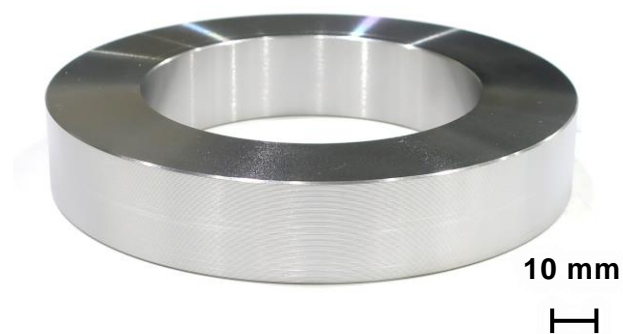
Fig. 2-4 Appearance of sample cooled in nitrogen atmosphere after carburizing.
