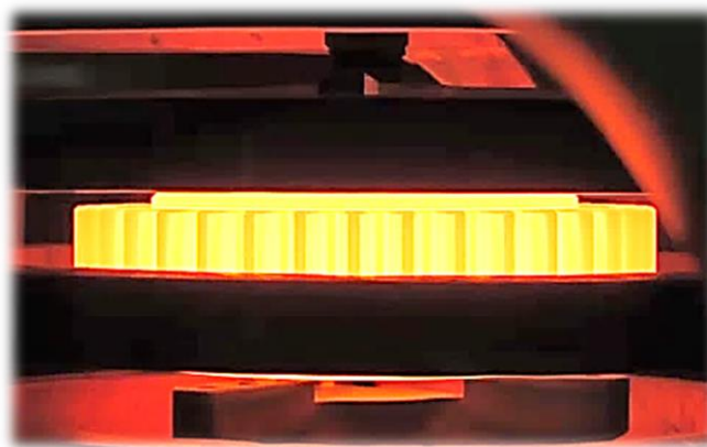
Fig. 1-6 Appearance of gear during heating using induction heating.
