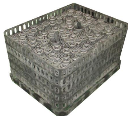
Fig. 1-3 appearance of the parts mounted on the basket jig for batch process.
