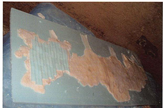
Fig. 31 Polystyrene as an intervention layer.
