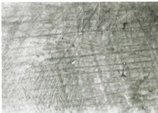
Fig. 3 The compression cracks in the paint layer made by a special tool (Black-and-white image)
