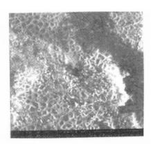
Wacker OH 290 was an effective polymer in consolidating the sandy limestone samples which homogenously penetrated into these samples forming net chains without causing any changes in the original color of these samples.
