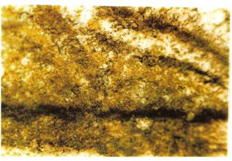
A SEM electron micrograph showed fungal species that had deeply penetrated into these blocks and caused serious damage to the mineral constituents and the physical structure of limestone.
