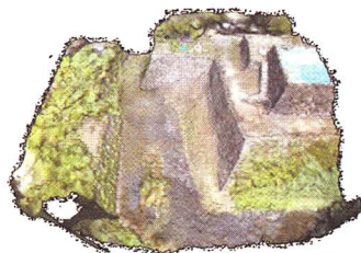
Fig.2 Reconstructed 3D surfaces of the site with MVS based on SfM output. 1.3M faces model is simplified to 0.09M faces to apply the proposed method.
