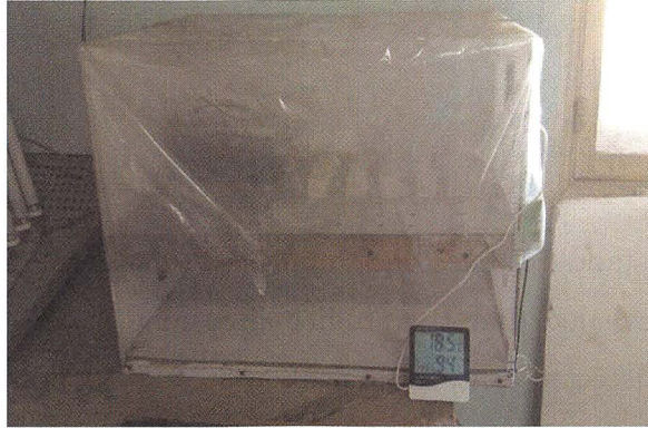
Fig. 4 Photograph showing that the percentage humidity in the test system was 90%
