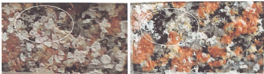
Fig. 13 Results of AB57+EDTA 10% after 72h
