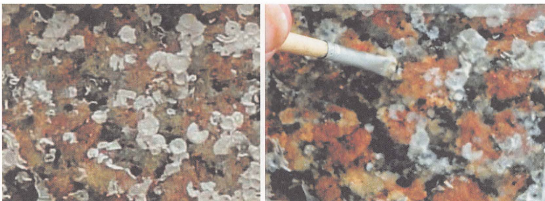
Fig. 7 Results of AB57+EDTA 20% after 48h
