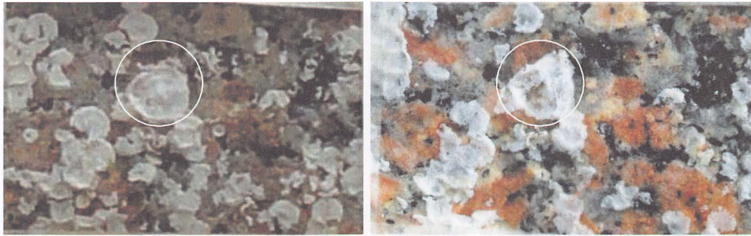
Fig. 8 Results of EDTA 10% after 48h
