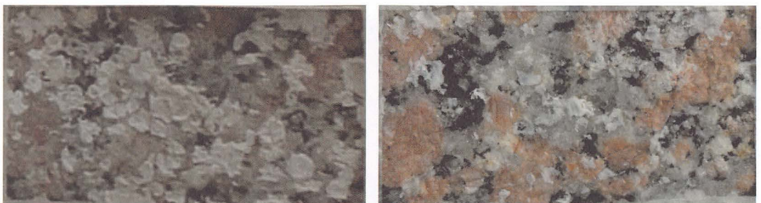
Fig. 17 Results of AB57+EDTA 10% after seven days
