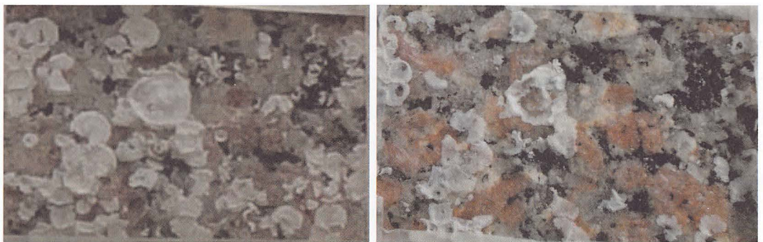
Fig. 16 Results of EDTA 10% after seven days
