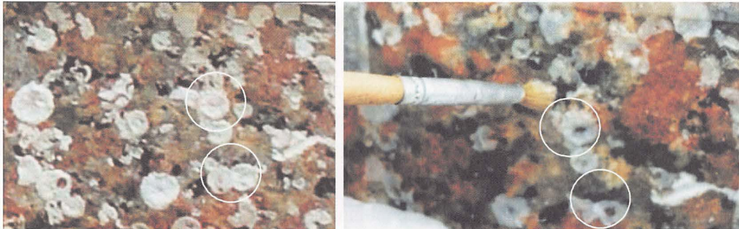
Fig. 5 Results of EDTA 20% after 24h
