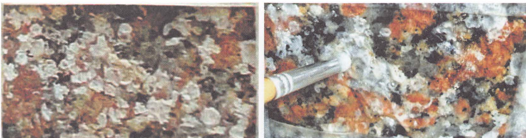
Fig. 9 Results of AB57+EDTA 10% after 48h during cleaning with a short-haired brush
