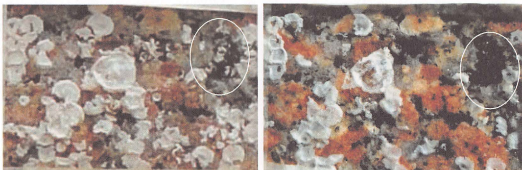
Fig. 12 Results of EDTA 10% after 72h
