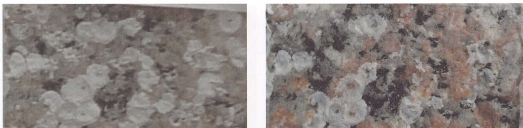
Fig. 18 Results of EDTA 5% after seven days
