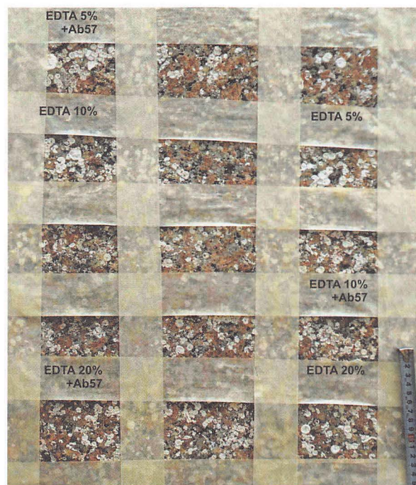
Fig.4 Showing the areas of the applied six poultices
