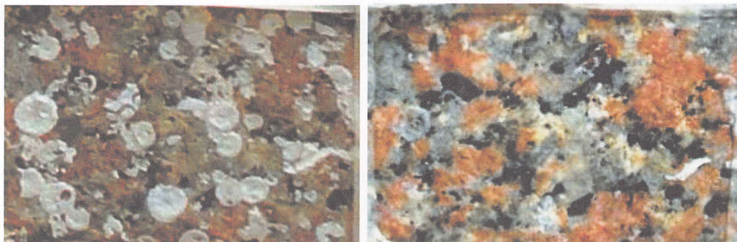
Fig. 10 Results of EDTA 20% after 72h
