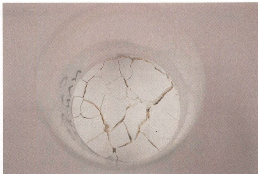
Fig. 6 Solidification of Nanorestore and CaCO 3 mixture (Nanorestore と CaCO 3 の混合物の固化性)
