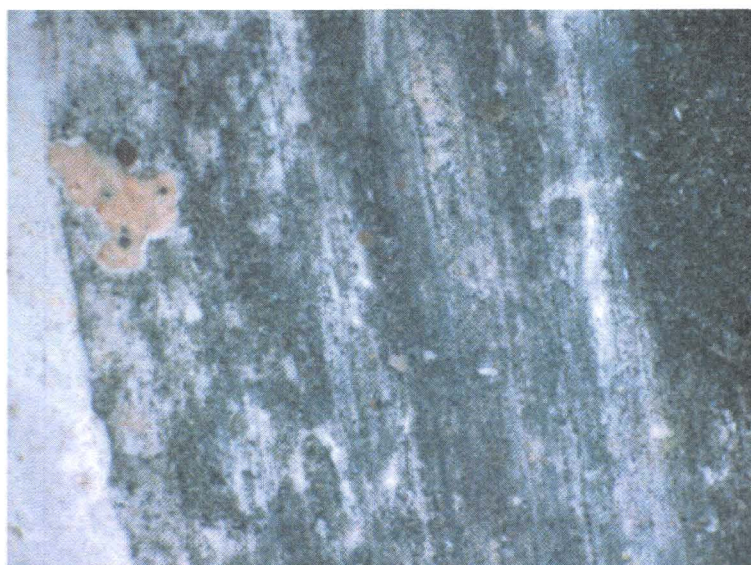
Fig. 13 Microscopic view of grey pigments (black carbon applied over white plaster)
