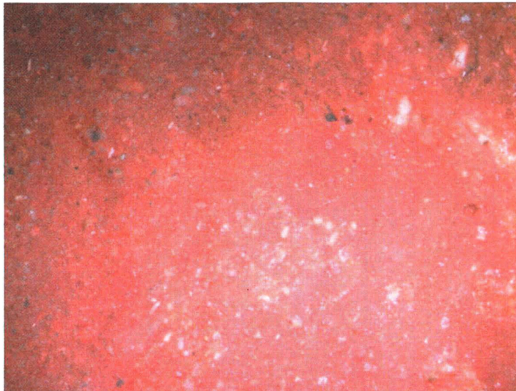
Fig. 11 Microscopic view of red pigments (massive granular aggregate particles appear to be uniform)
