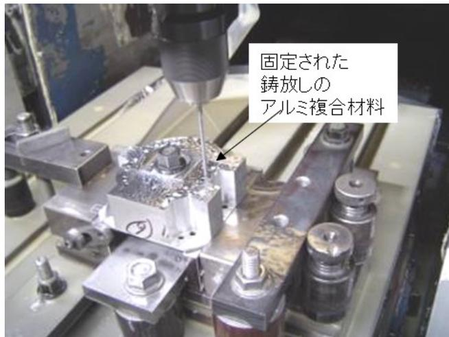
Fig. 6-13 Photograph of rotor housing in the process of end milling.
