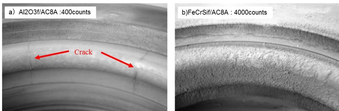
**Fig. 6-21** Appearance of crack at piston head lip after thermal shock test.
