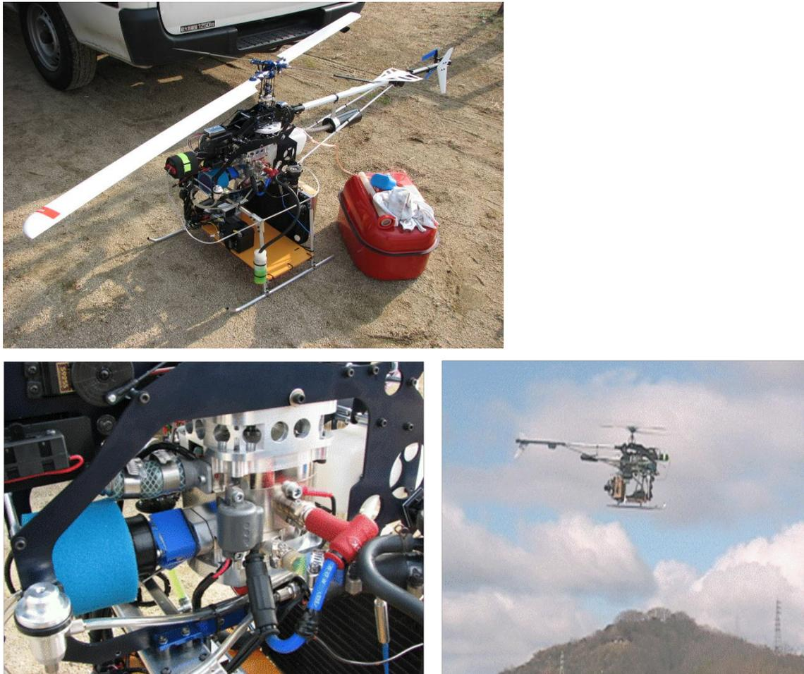
**Fig. 6-18** Photos of the flight test of the small unmanned helicopter equipped with the REheli.
