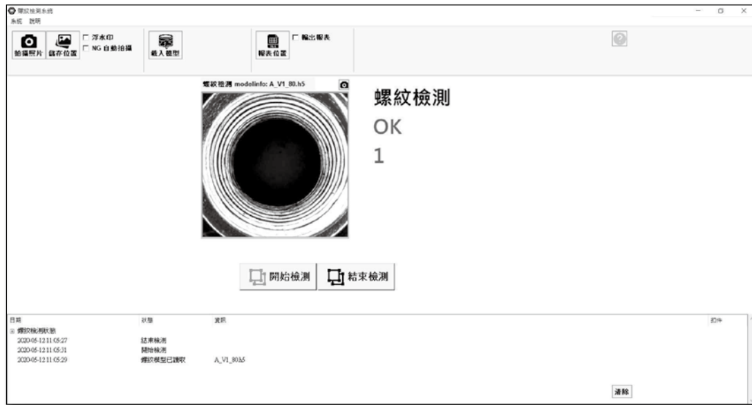
Fig. 4.2 User interface of a customized machine vision system.
