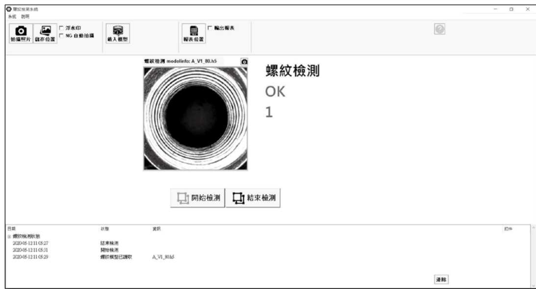
Fig. 5.1 Inspection results for a normal internal screw nut.
