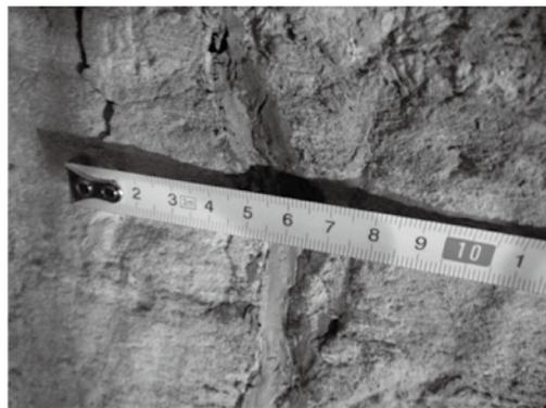
**Fig. 10** Status of crack filled with cement slurry
