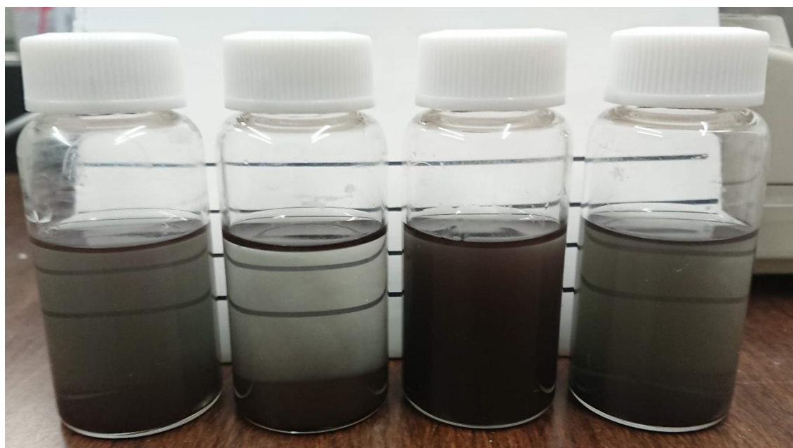
Fig. 3 Example of dispersion stability evaluation experiment results (From the left, DMSO, THF, GBL and methanol)
