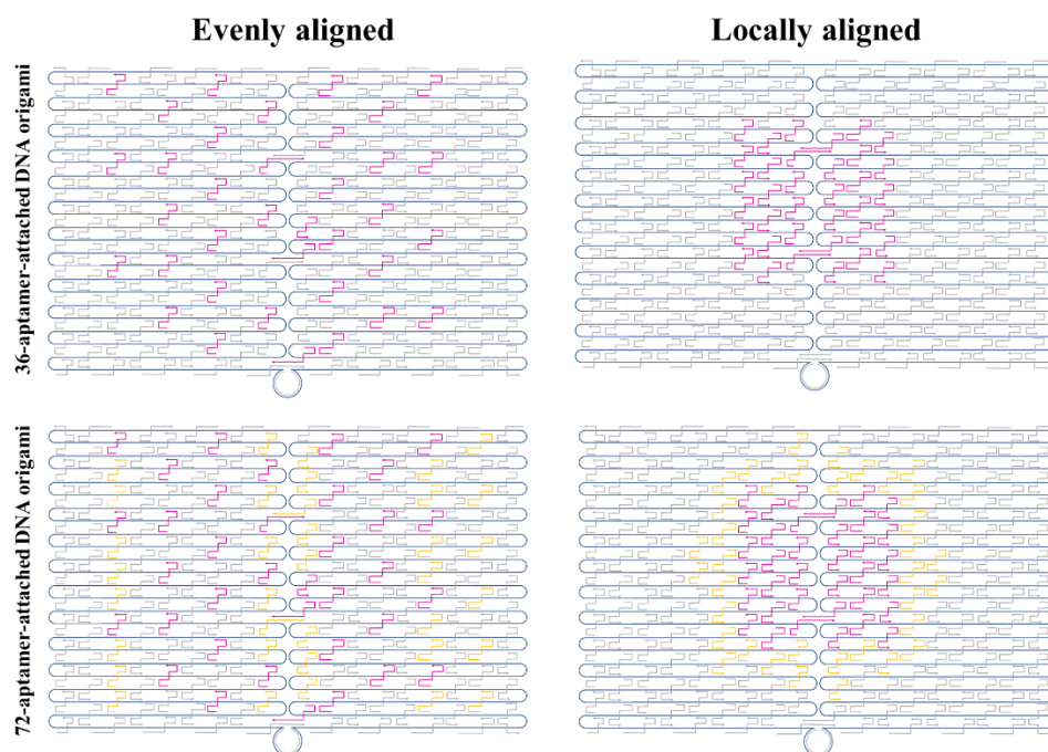
Fig. 5-10 A comparison of redesign of 72 aptamer-attached DNA origami. The position of aptamer was indicated by colored symbol: pink shows the positions of 36 aptamer and both of orange and pink shows the positions of 72 aptamers.
