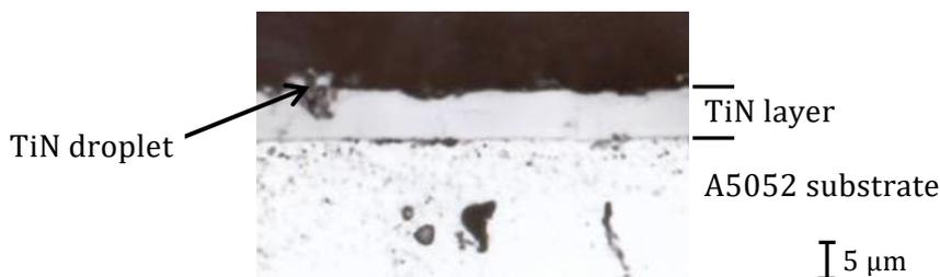
Fig. 2.29 Cross-sectional fractures of the TiN films deposited by AIP method.
