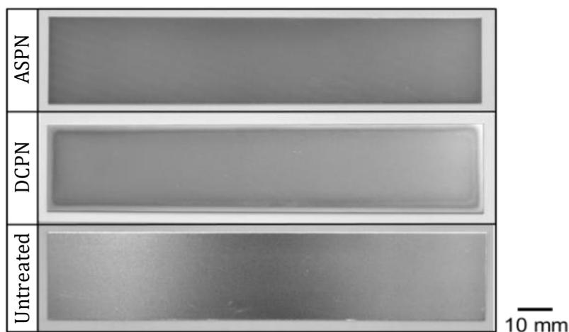
Fig. 6.3 Appearance of untreated and nitrided SUS304.
