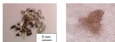
Figure 1. Photographs of Ti–Pd turnings (left) and Ti–Pd(Hy) powder (right).
