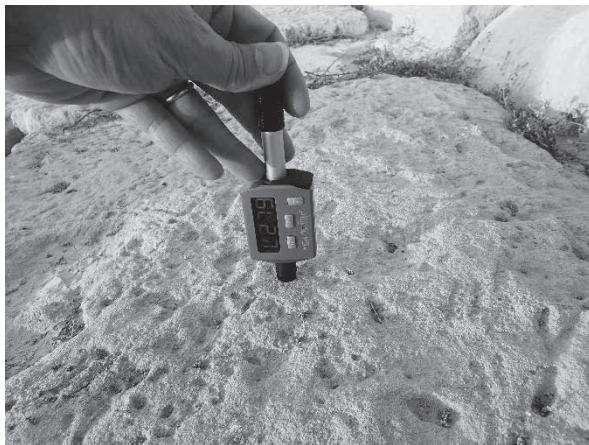
Fig.17 Measuring technique with rebound type hardening meter
