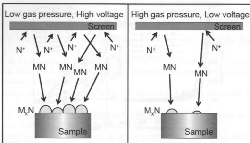
Fig. 6 Schematic illustration of mechanism of nitrogen mass transfer in ASPN.
