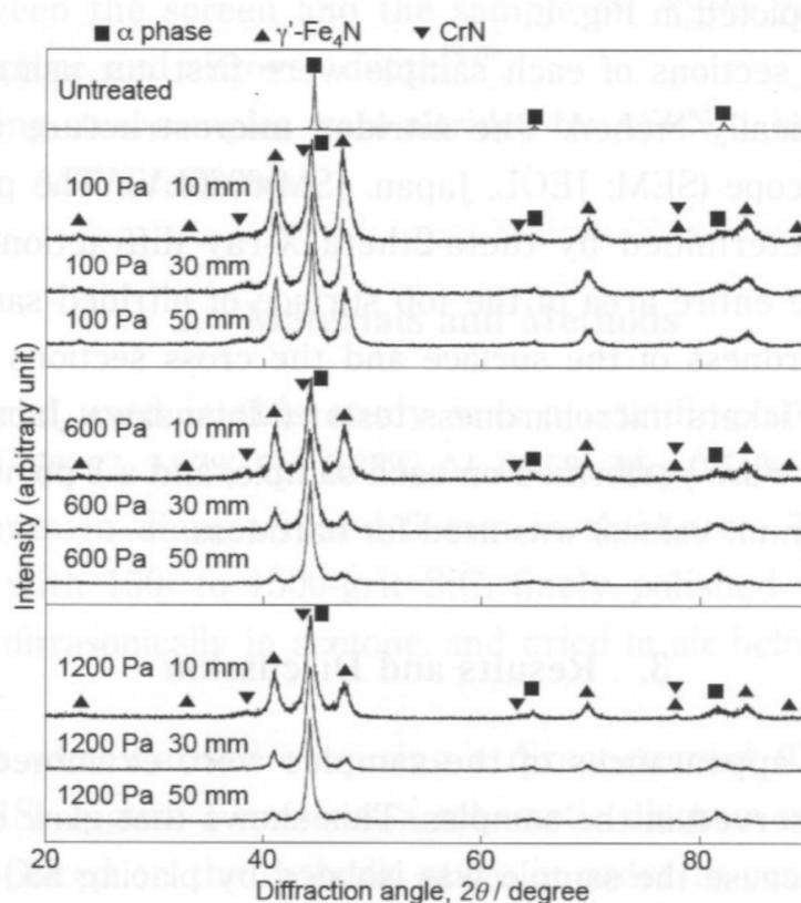
Fig. 3 XRD pattern of SACM645 sample treated by ASPN at 823 K for 18 ks.
