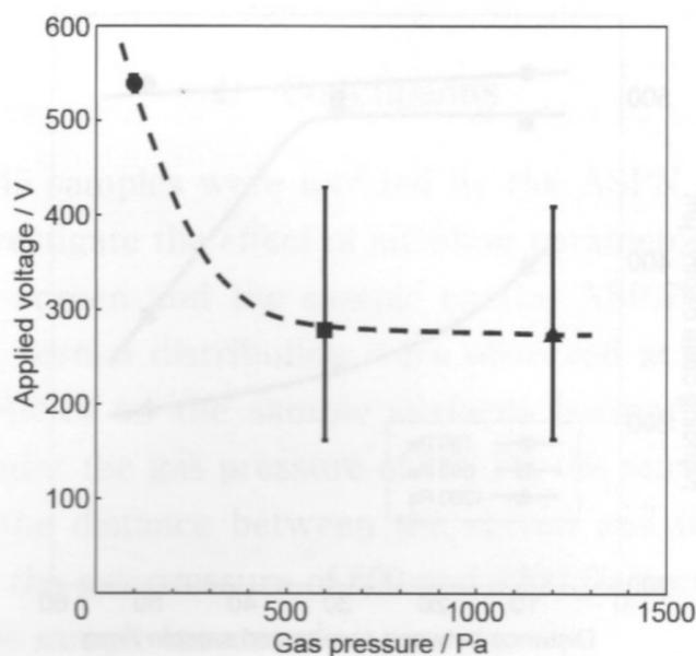
Fig. 5 Relationships between applied voltage and gas pressure of SACM645 sample treated by ASPN at 823 K for 18 ks.
