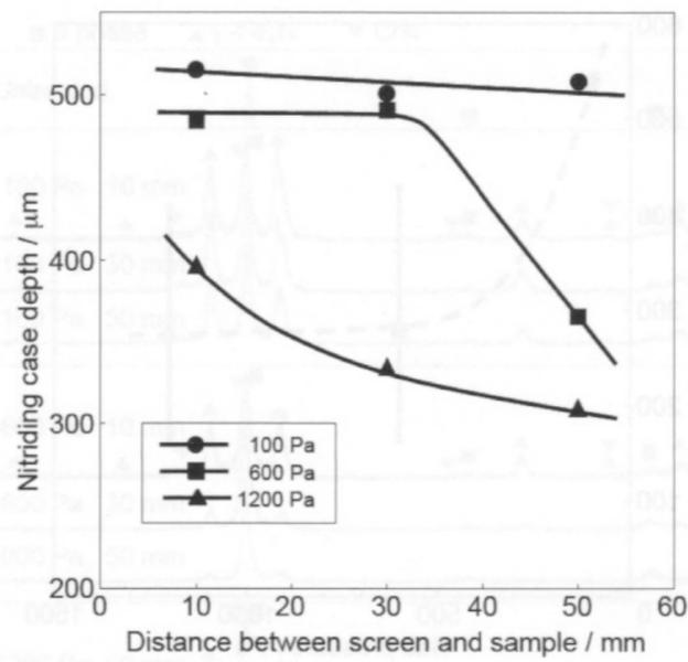
Fig. 7 Nitriding case depth of SACM645 sample treated by ASPN at 823 K for 18 ks.
