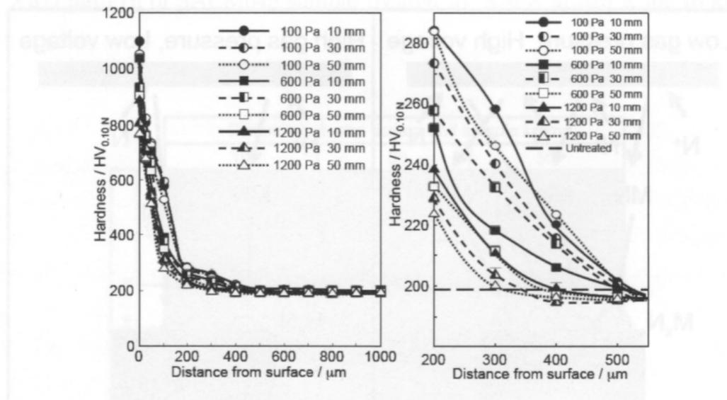
Fig. 8 Hardness distribution from surface of SACM645 sample treated by ASPN at 823 K for 18 ks. (a) from 0 to 1000 μm and (b) from 200 to 550 μm.
