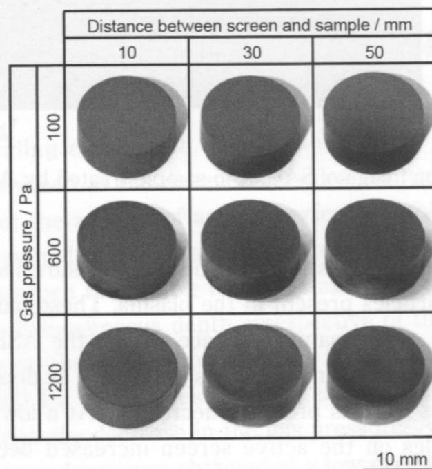
Fig. 2 Appearance of SACM645 sample treated by ASPN at 823 K for 18 ks.
