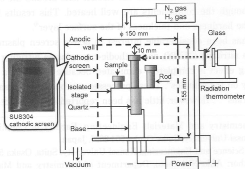
Fig. 1 Schematic illustration of ASPN furnace.
