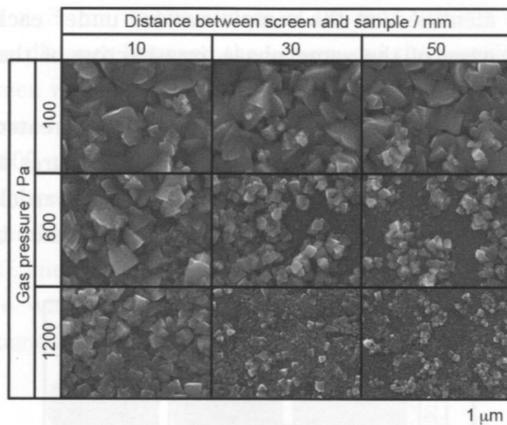
Fig. 4 Secondary electron image of SACM645 sample treated by ASPN at 823 K for 18 ks.
