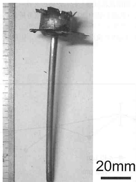
Fig. 3 Appearance of an extruded brass rod at 773 K.
