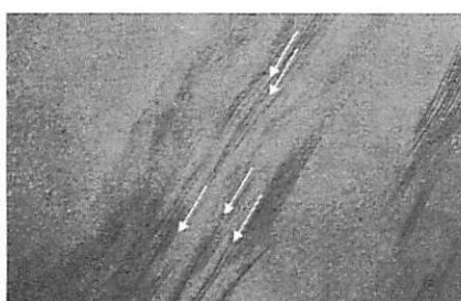
Fig.6 TEMs of the epoxy / tertiary-amine organoclay nanocomposites (Clay content: 5 wt%) cured at 130 °C.
