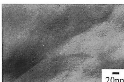
Fig.6 TEMs of the epoxy / tertiary-amine organoclay nanocomposites (Clay content: 5 wt%) cured at 130 °C.
