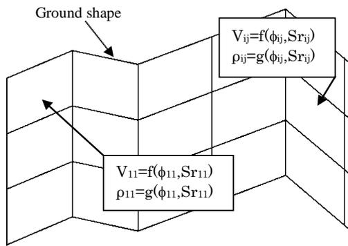
Figure 4. The cell-based rock mass model for conversion calculations
