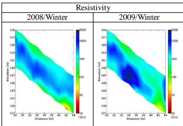
Figure 7. Results of electric prospecting
