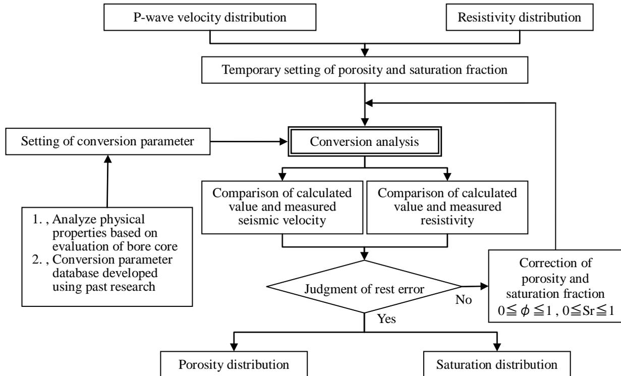
Figure 5. System flow for evaluation of geological structure using the conversion method
