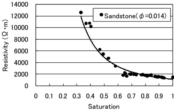
Figure 8. Example of relationship between resistivity and saturation
