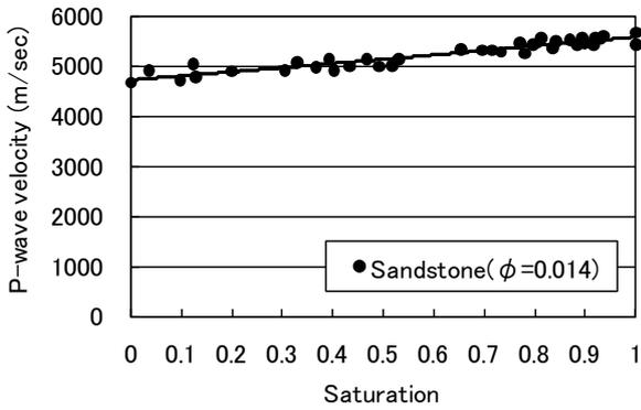
Figure 9. Example of relationship between P-wave velocity and saturation
