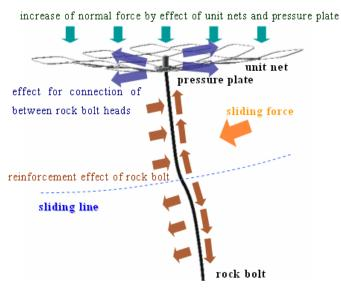
Fig.2 Reinforcement mechanism of this slope stability method
