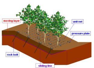
Fig.1 Concept of this slope stability method
