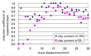
Fig.6 Relations between shear displacement and reduction coefficient of supported slope
