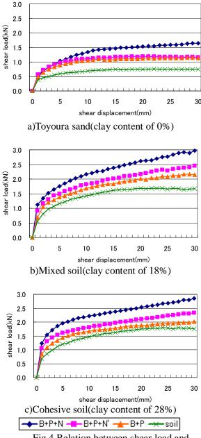
Fig.4 Relation between shear load and shear displacement
