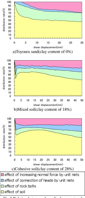
Fig.5 Relation between shear displacement and distribution ratio of each reinforcement effects
