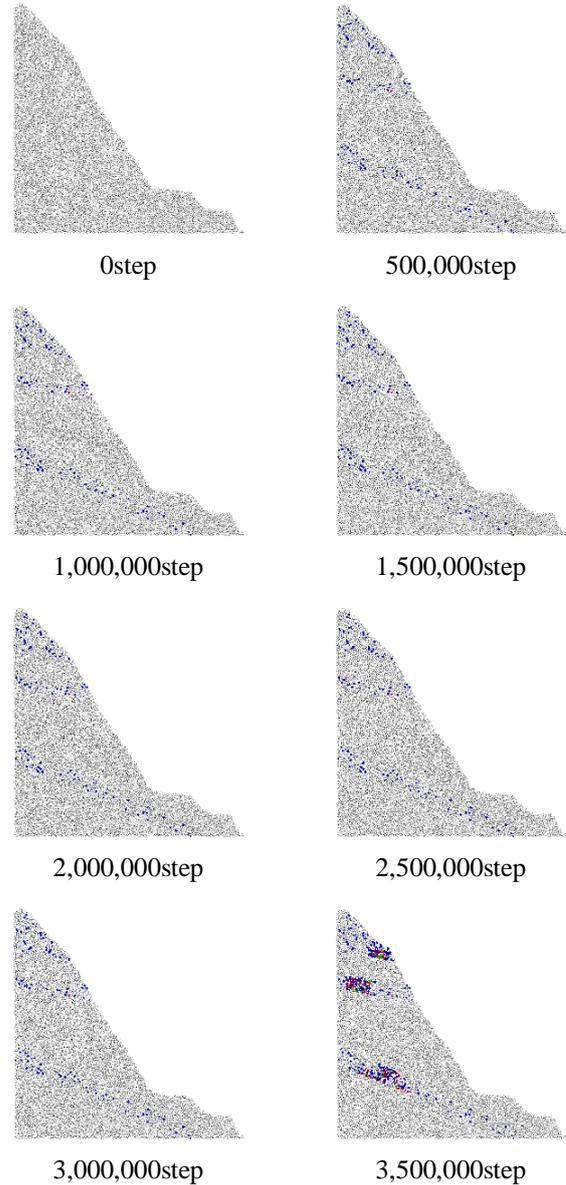
Figure 8. The development of the fracture
