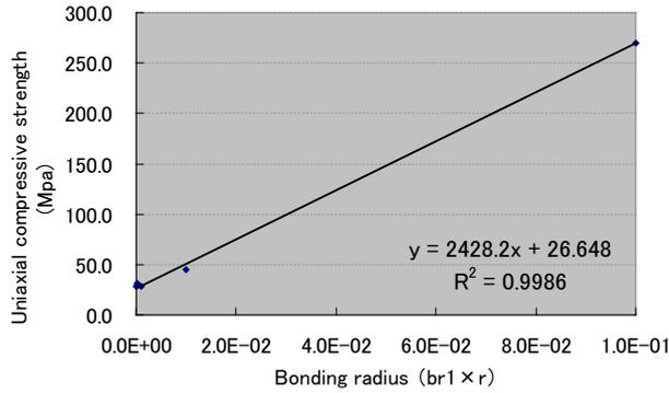
Figure 6. The relation between bonding radius and uniaxial compressive strength
