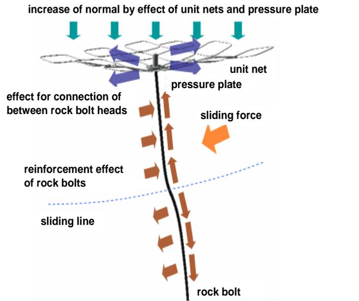
Fig.2 Reinforcement mechanism of this slope stability method
