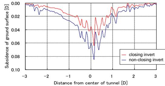
Figure9. The shape of subsidence of ground surface
