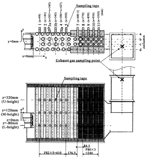
Fig. 2 Cross-section of test boiler
