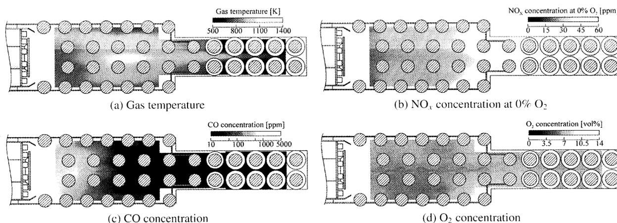
Fig. 5 Distribution of gas temperature and gas concentrations at U-height
