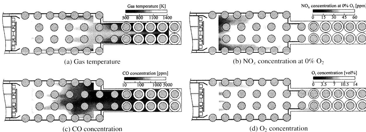
Fig. 3 Distribution of gas temperature and gas concentrations at L-height
