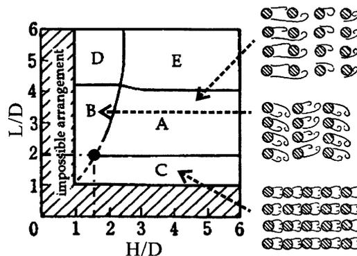
Fig. 7 Flow pattern map in tube-bank (uniform flow)<sup>(4)</sup>
