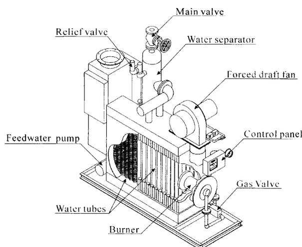
Fig. 1 Tube-nested combustor
