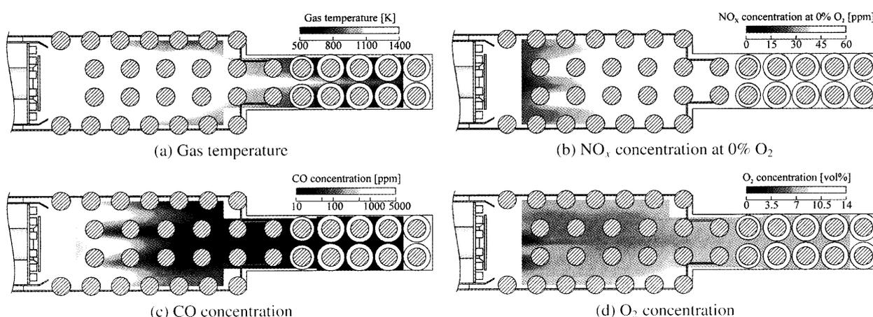
Fig. 4 Distribution of gas temperature and gas concentrations at M-height
