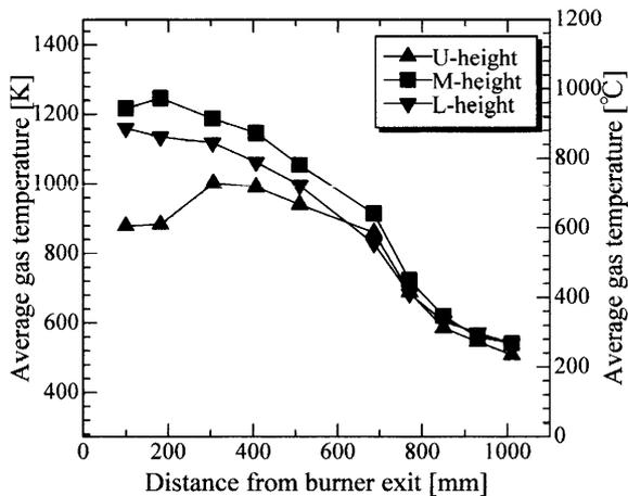
Fig. 8 Longitudinal distribution of average gas temperature
