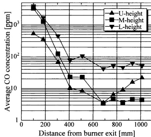
Fig. 10 Longitudinal distribution of average CO concentration
