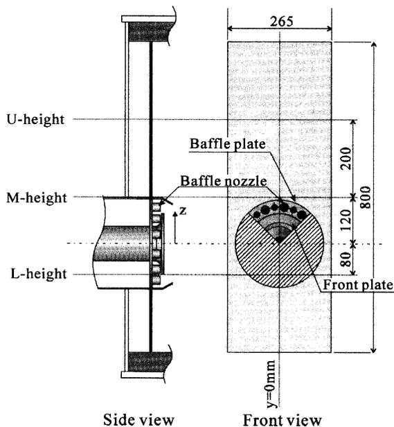
Fig. 6 Burner and measuring height
