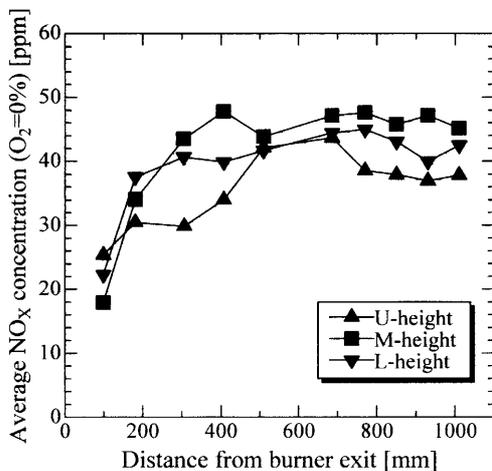
Fig. 9 Longitudinal distribution of average NO<sub>x</sub> concentration (at 0% O<sub>2</sub>)
