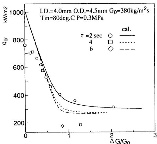
Fig. 8 CHF under the oscillatory flow condition
