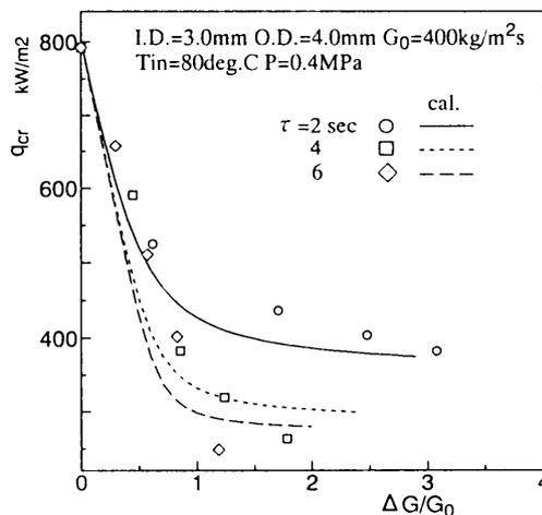
Fig. 6 CHF under the oscillatory flow condition
