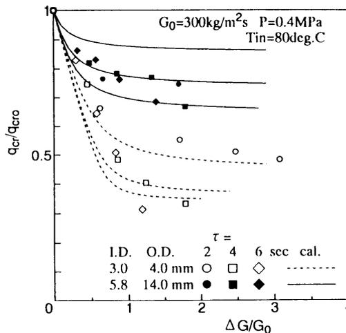
Fig. 11 Influence of the tube wall heat capacity on the CHF
