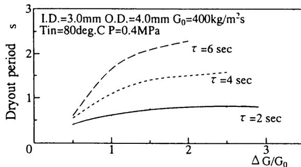
Fig. 7 Simulation results of the dryout period at the tube exit
