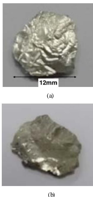
FIG. 2 SINTERED METAL PASTE. (A) FE AND (B) AL
