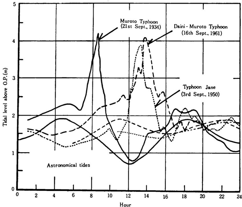
Fig. 8 Observed tidal curves in Osaka.
