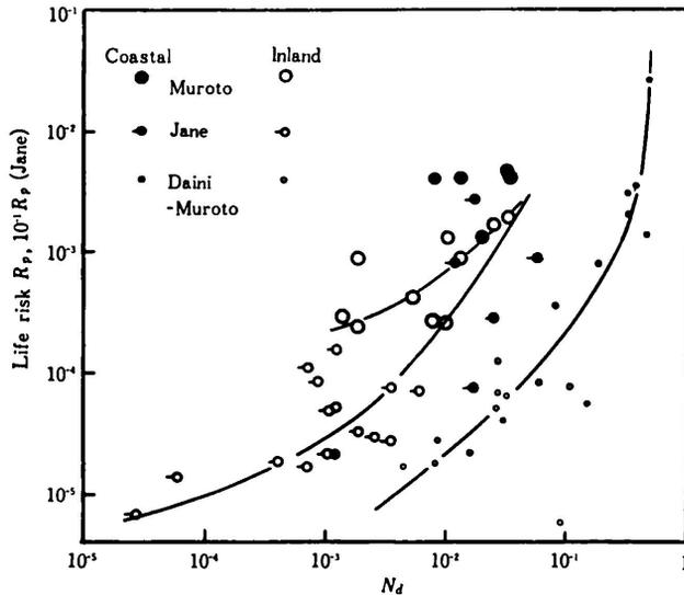
Fig. 16 Relationship between the ratio of houses damaged and the life risk that includes injured persons.
