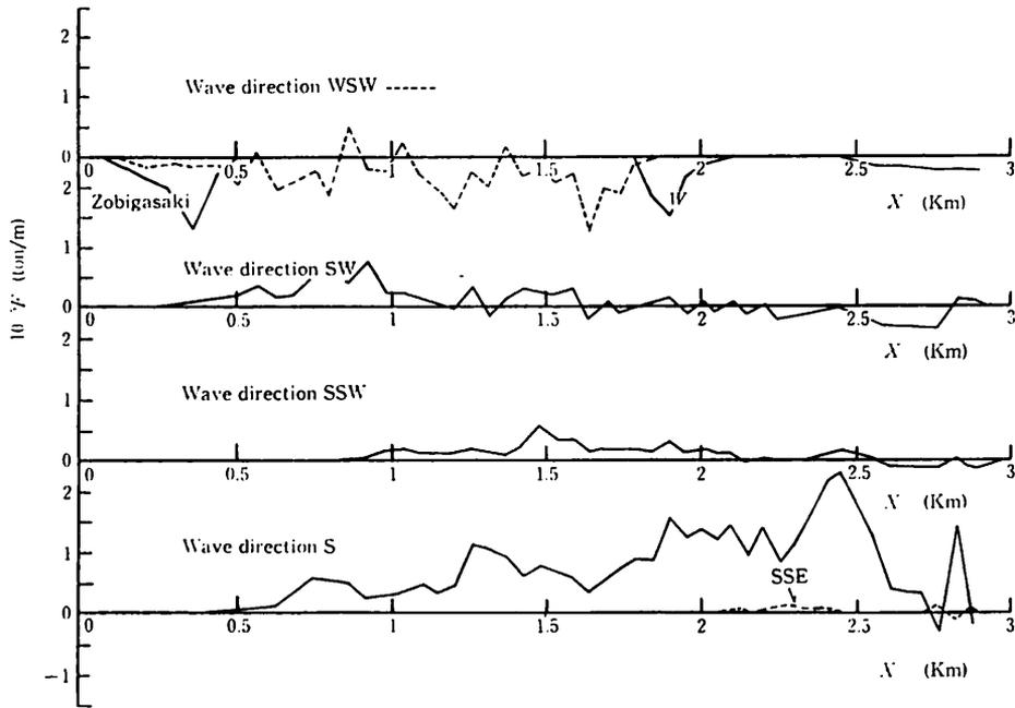
Fig. 27 Contributions of longshore wave energy flux in each predominant wave direction to the total one.
