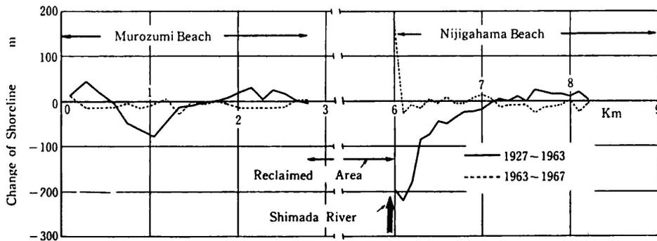
Fig. 5 Changes of shorelines with the distance measured from Zobigasaki headland.
