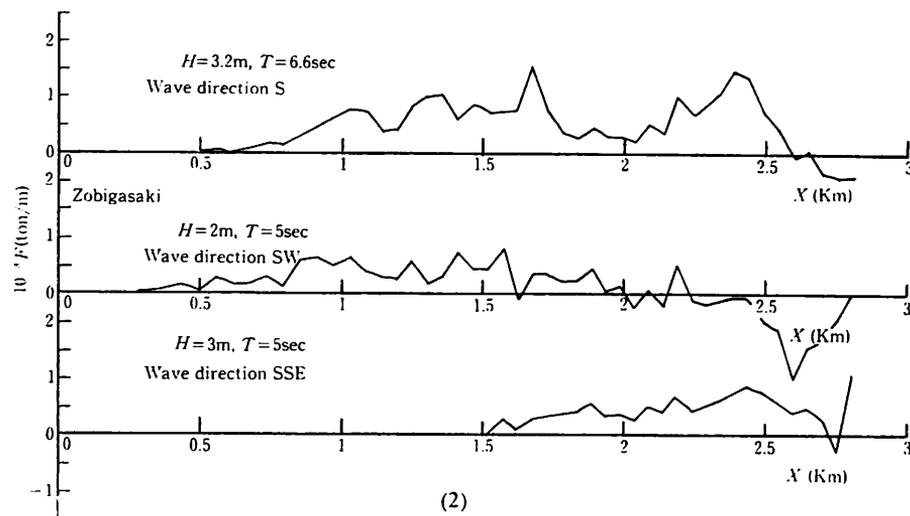
Fig. 32 Distributions of longshore wave energy flux derived from the likely maximum wave in each approaching direction.
