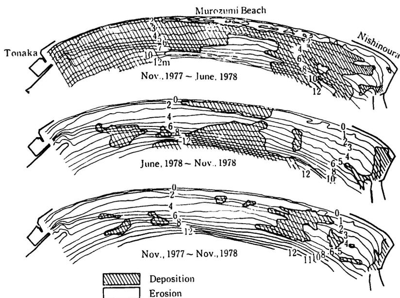
Fig. 7 Areas of erosion and deposition based on the data from hydrographic survey.
