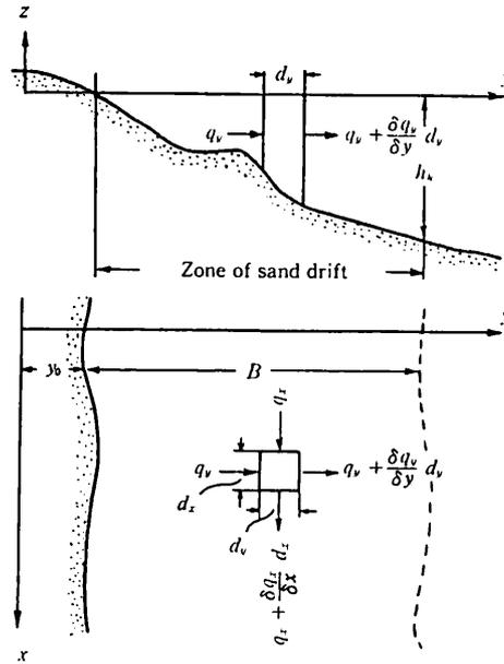
Fig. 24 Co-ordinate system used for predicting shoreline changes [6].
