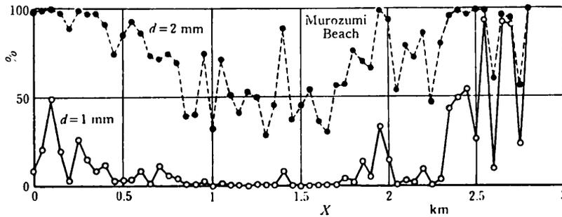
(c) Percent of sediments less 1 mm or 2 mm in diameter
