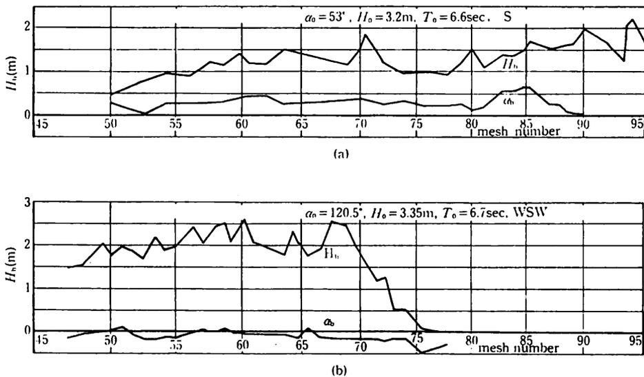
Fig. 33 Distributions of wave height and wave direction at breaking point along Murozumi beach.
