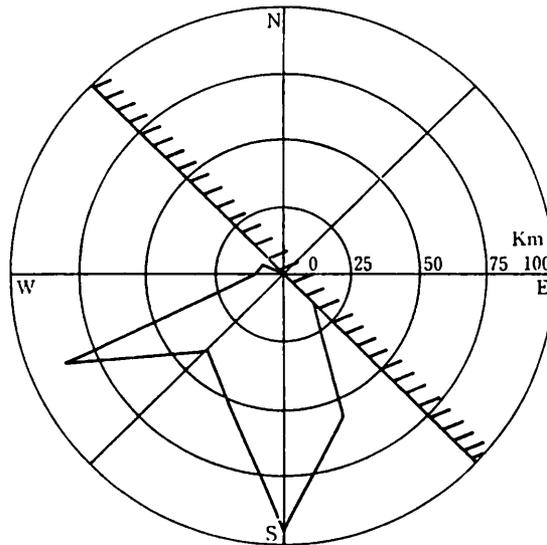
Fig. 10 Maximum fetch in each direction from Murozumi beach.
