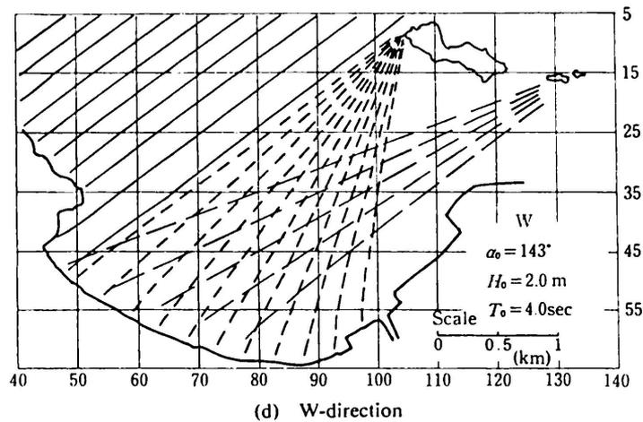
Fig. 16 Examples of wave refraction-diffraction diagrams, representing various directions of wave approaching (Numbers on the co-ordinates show mesh number in calculation).
