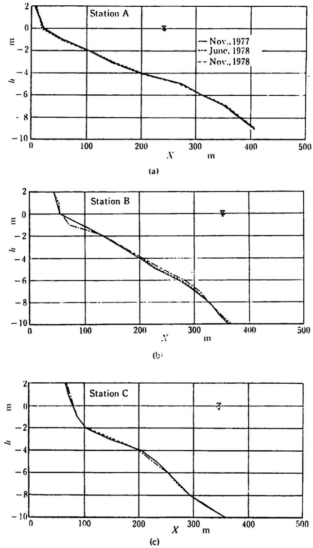
Fig. 6 Comparison of beach profiles at various stations along Murozumi beach (Locations of A, B and C are shown in Fig. 4).
