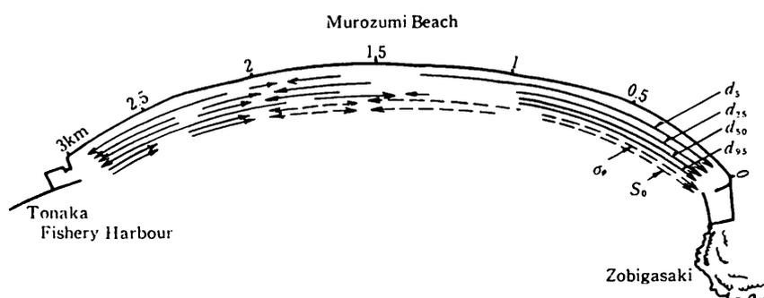
Fig. 21 Schematic diagram of directions of longshore sediment transport.
