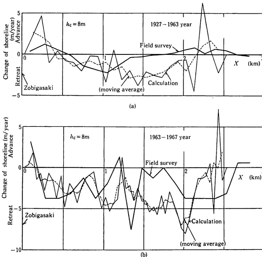
Fig. 29 Comparison on shoreline changes between results of numerical simulation and field survey.
