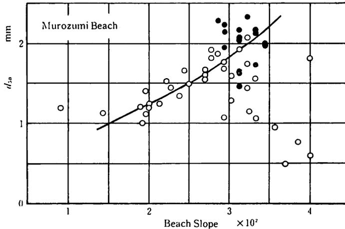
Fig. 20 Beach slope versus median diameter of sediments.
