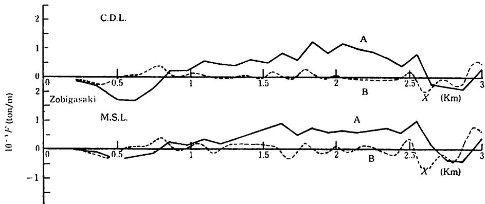
Fig. 28 Averaged annual longshore wave energy flux before reclamation (Stage I).
