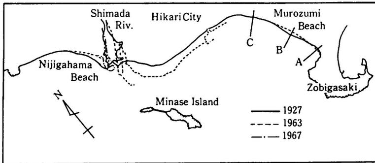
Fig. 4 Comparison of shoreline configurations.
