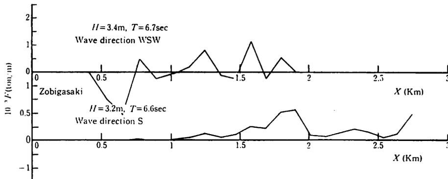
Fig. 34 Distributions of longshore wave energy flux derived from condition within Stage I.
