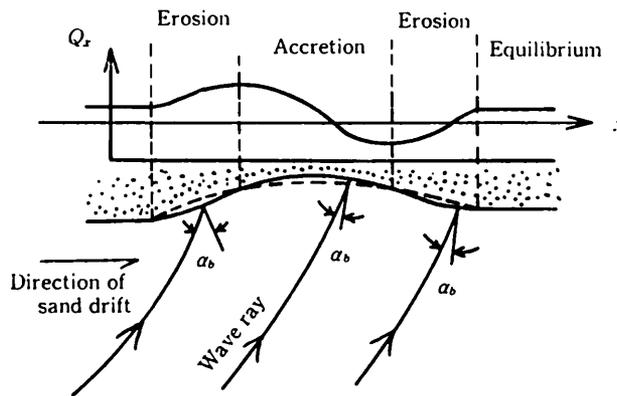
Fig. 25 Schematic diagram of beach changes [6].
