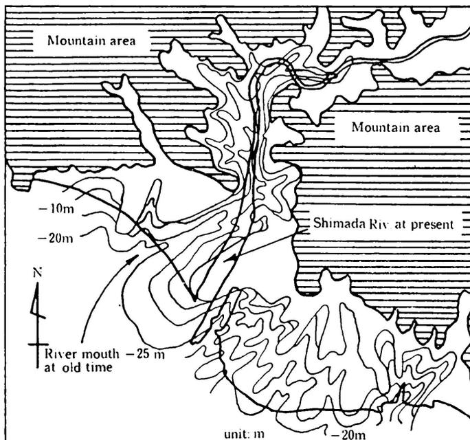
Fig. 2 Depth sounding chart in the vicinity of the mouth of the Shimada river.
