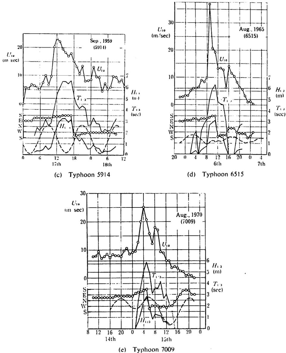
Fig. 13 Changes of wave characteristics as a function of time predicted by the S.M.B. method.
