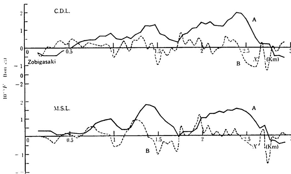
Fig. 26 Averaged annual longshore wave energy flux after reclamation (Stage II).
