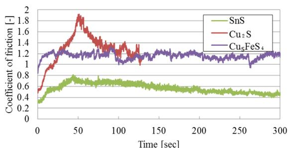
Fig.7 Results of friction test
