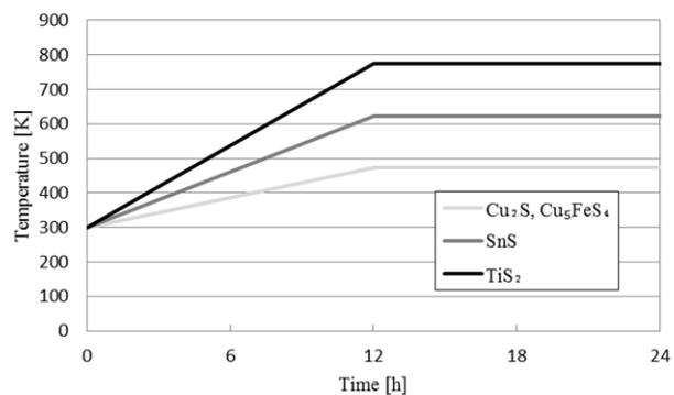
Fig.2 Synthesis temperature and time
