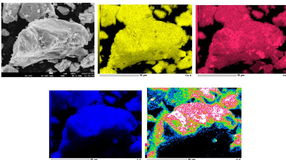
Fig.4 EDS results of synthesized Cu<sub>5</sub>FeS<sub>4</sub> (bornite)
