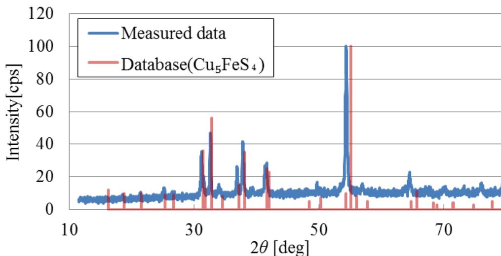
Fig.3 X-ray diffraction results of Cu<sub>5</sub>FeS<sub>4</sub>
