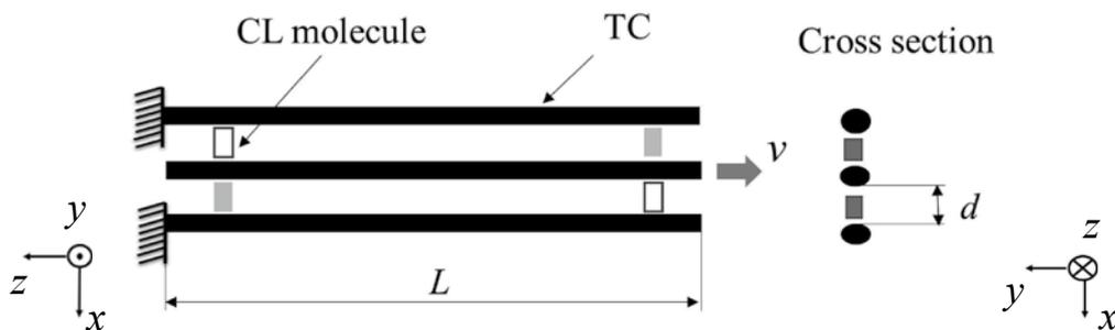
Fig. 3 Schematic of the tensile simulation model (4 Cross-Links)
