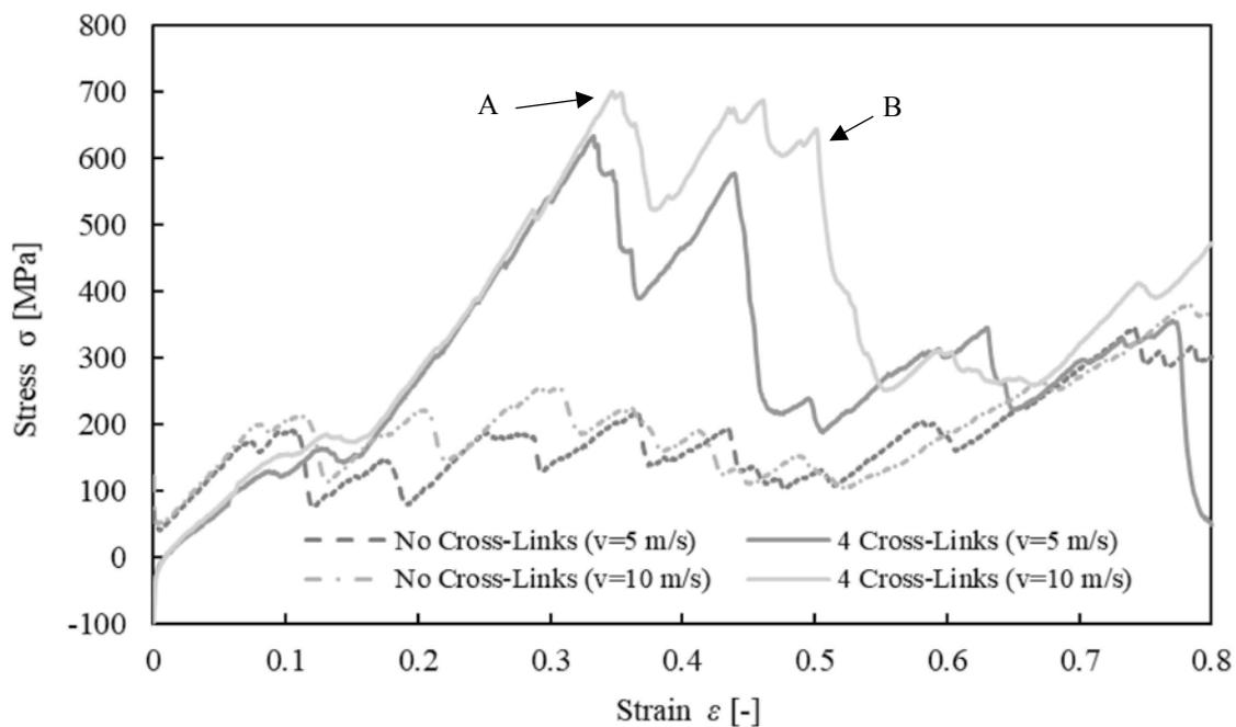
Fig. 7 Stress-strain curves for 4 Cross-Links and No Cross-Links models
