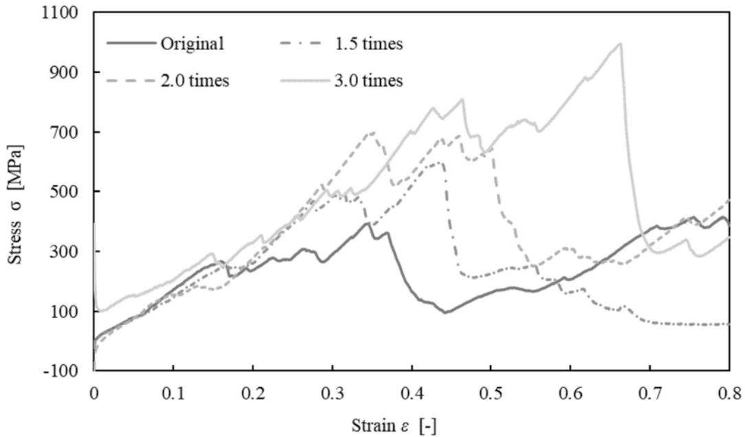
**Fig. 5** Change in stress among the different electric charges of hydrogen atoms in CL molecules
