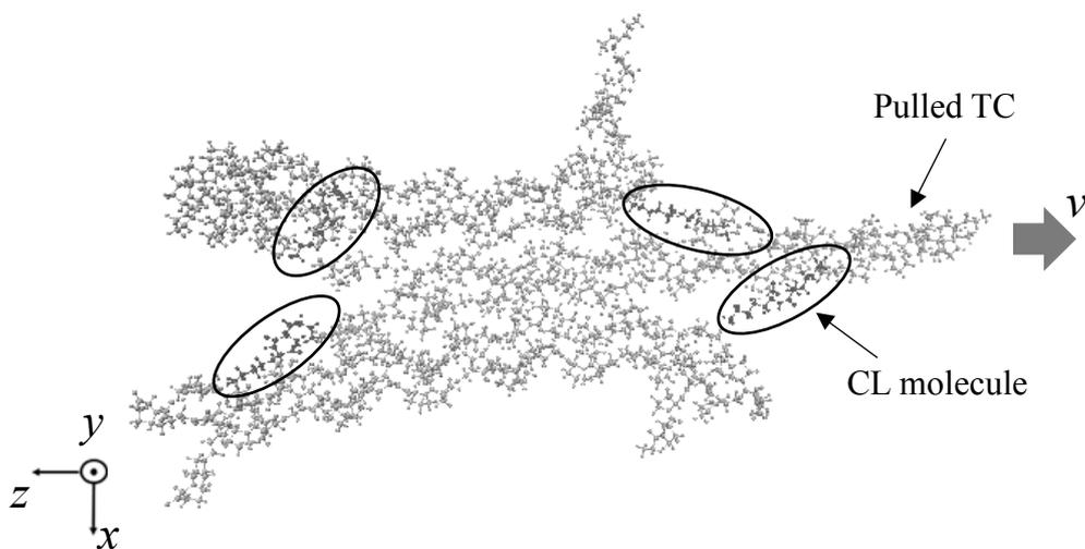
Fig. 8 Snapshot obtained by tensile simulation (at point A in Fig. 7,  $v = 10$  m/s)
