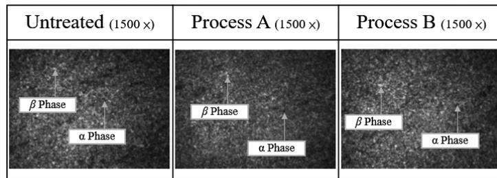
Figure 2. Microstructures for different cryogenic treatment processes
