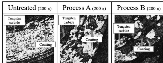
Figure 1. Observed surface after the wear resistance test
