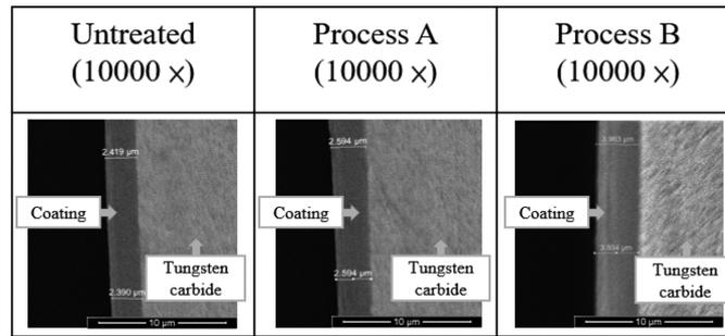
Figure 4. Adhesion between tungsten carbide and coating
