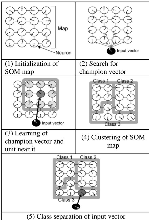
Figure.8 The basis of the algorithm of SOM
