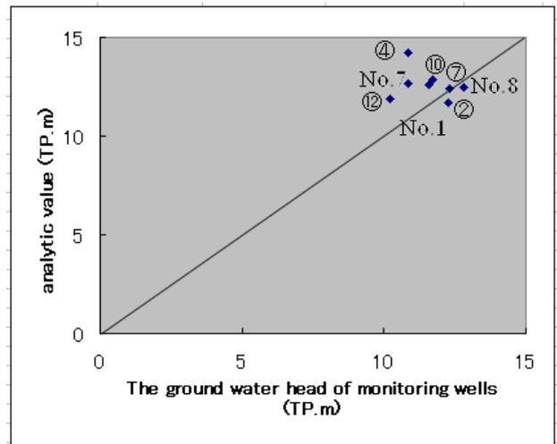
Fig14. Comparison between values measured and the predictions of the analysis
