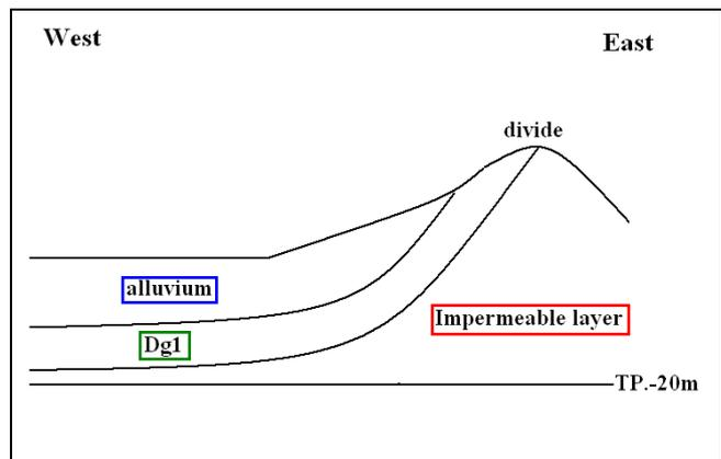
Fig.4 Conceptual diagram of the model
