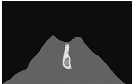
図2 薩摩硫黄島の計測結果 [8] Fig. 2. Muography image of the Satsuma-Iwojima. [8]
